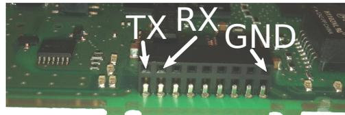
Figure 1: UART send and receive signals that can be used to interact with the PLC.
