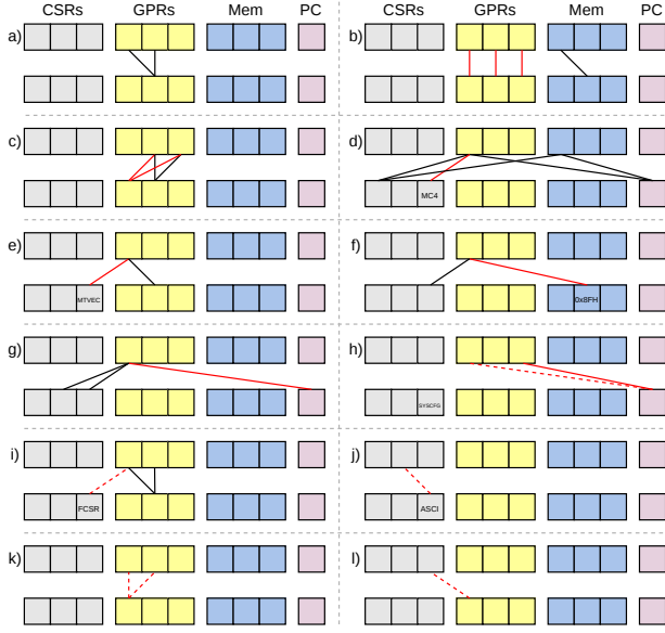
Figure 2: Architectural IFs from top (before instruction execution) to bottom (after instruction execution). The boxes represent architecturally visible state elements: Control and Status Registers (CSRs), General Purpose Registers (GPRs), memory (Mem) and the Program Counter (PC). Solid black lines are expected architectural flows. Dashed red lines indicate missing IFs. (a) Expected flow for an add instruction. (b) Intel’s erratum BV84 for a REP MOVSB instruction [35]. (c) A multiplication instruction in Ibex writes to the wrong destination [25]. (d) AMD’s erratum 699 for an VMLoad instruction [35]. (e) Kronos CVE 2023-51973 for an add instruction [25]. (f) Intel’s erratum AAT106 for a VMPTRLD instruction [35]. (g) AMD’s erratum 1321 for a WRMSR instruction [35]. (h) AMD’s erratum 721 [35]. (i) ProcessorFuzz bug 7 [27]. (j) BOOM issue 503. (k) VexRiscv bug CVE 2023-34896 [24]. (l) AMD’s erratum 719 [35].
